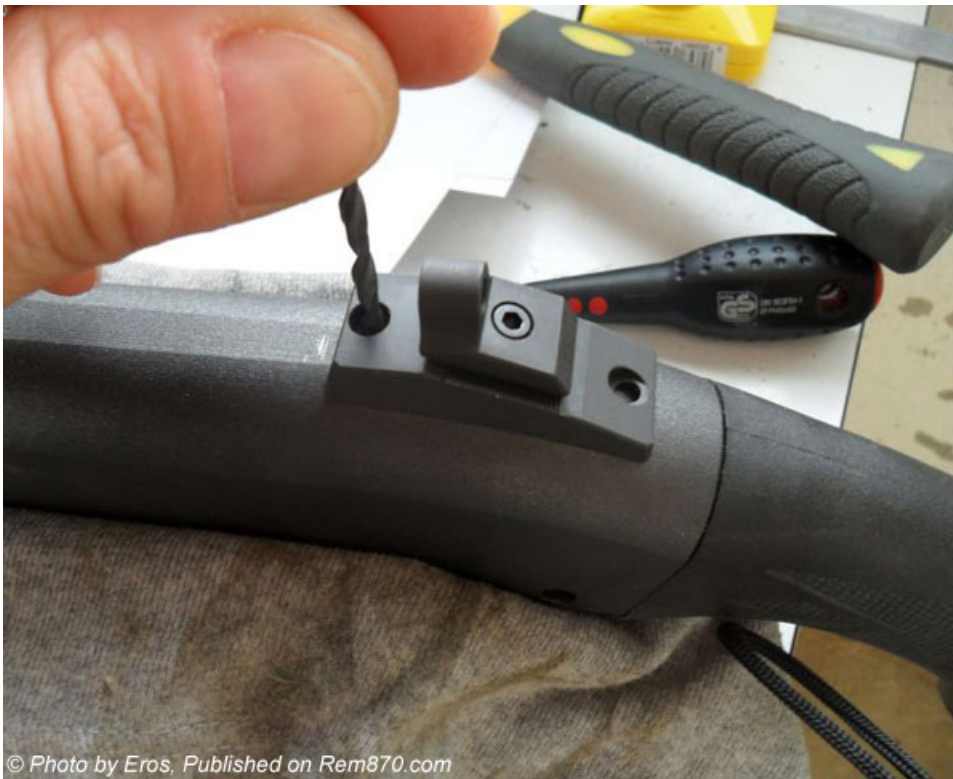
Here we see receiver drilling.
