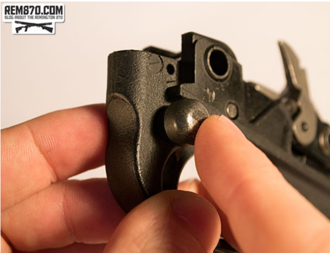
6. Remove the old safety button and install the new safety from the right side.
