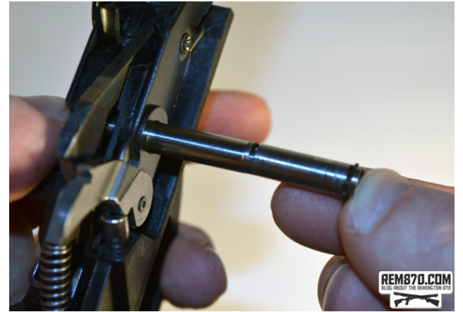
5. Use the second side of the Carrier Pivot Slave Pin to insert the carrier tube back into place.
