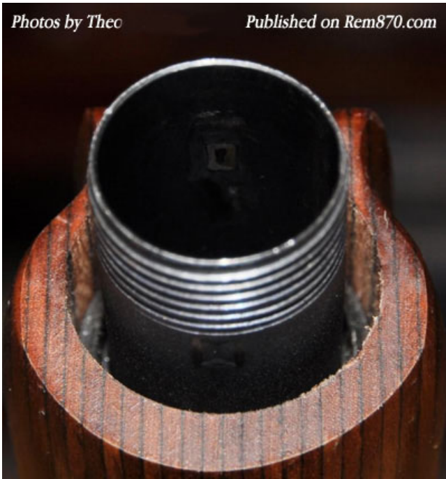
Un-blued finished tube Inside (after dimple removal).
