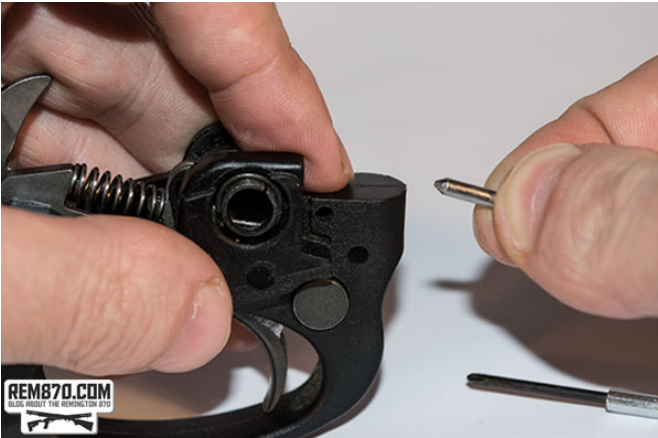
4. Take out the safety switch retaining pin.
