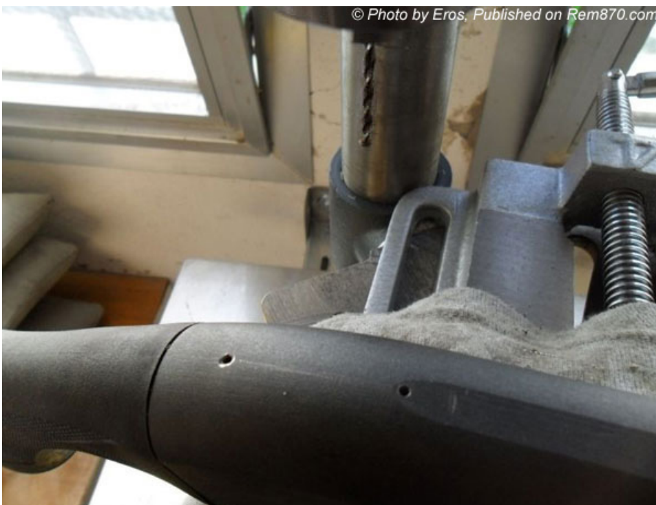
This shows the final drilled receiver.
