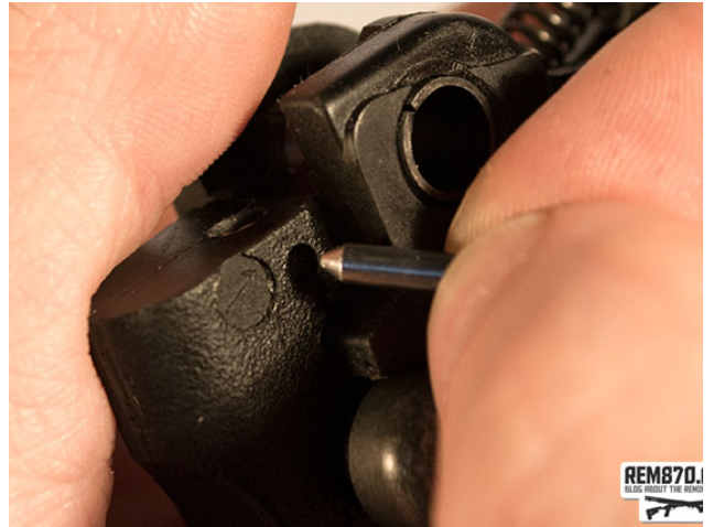
9. Insert safety switch pin with the pointed end first.
