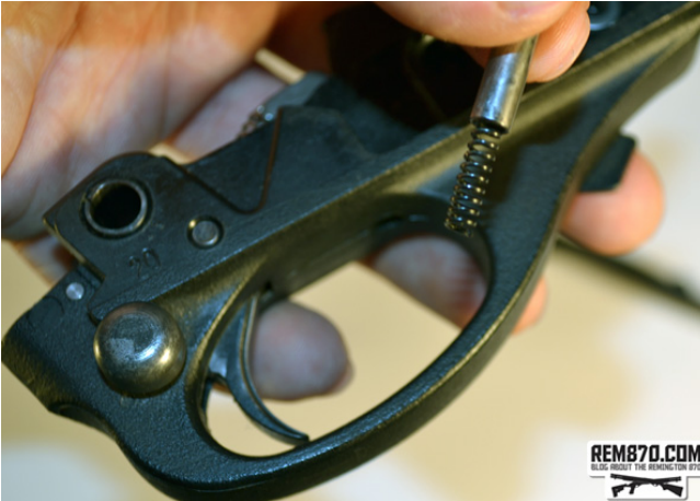
4. Insert the new Carrier Dog Follower Spring and reverse the process
