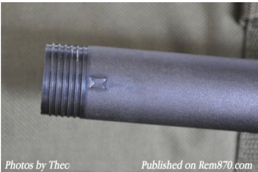
To the left is the outside of a blued finished tube.
