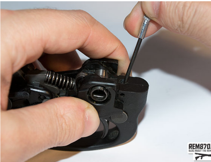
10. Depress the safety detent spring into the safety detent channel and insert the retaining pin.
