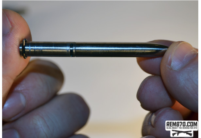
5. Use the second side of the Carrier Pivot Slave Pin to insert the carrier tube back into place.
