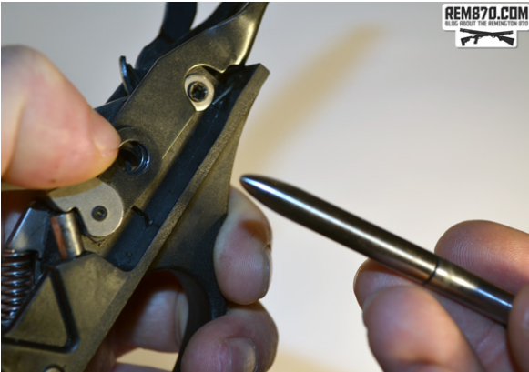
4. Insert the new Carrier Dog Follower Spring and reverse the process
