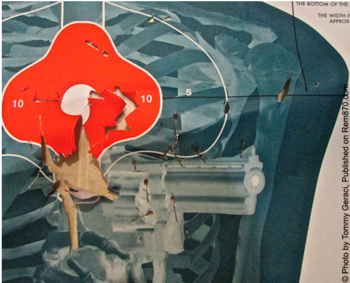
The Flechettes have an overall spread of 19X10" at 15 feet. Other than the enormous amount of spread, off camera the Flechettes pierced through a phone book proving it has tremendous penetrable capabilities.
